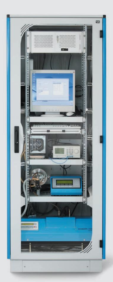
A proprietary automatic sample selection system allows up to 6 samples to be fed into the system. The factory juices to be analysed are selected by pneumatic means into the so called "reactor".
