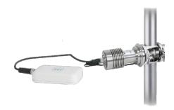
Important performance information such as cleanliness and humidity in the instrument are available on to your maintenance personal. At the same time, the instrument can communicate your production control via the trusted analog and serial interfaces or without cable via your factories W-LAN, saving effort of cabling.
